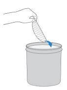
Clean the water inlet filter on the bottom of the Reservoir if it is clogged.
