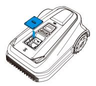
7. Tighten the screws on the inner cover.
