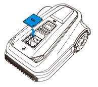
4. Insert the SIM card into the card tray with the metal side facing up, as shown in the image. Then, insert the card tray into the slot.
