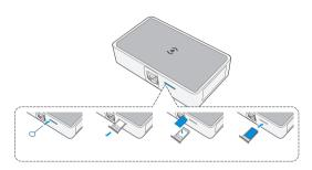
5. Connect the module connector to the cellular module, ensuring the connector is positioned with the "e" icon facing up. Arrange any excess cable neatly.
