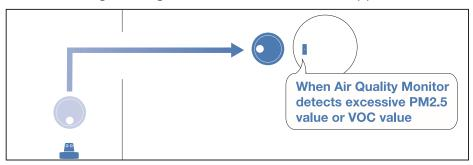
When both PM2.5 value and VOC value reach the standard, AIRBOT will automatically return to the charging dock.
