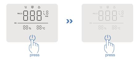
**Mobile Purification:** When AIRBOT is in Mobile Purification, press 1 to pause purification; Press 1 again to resume Mobile Purification.
