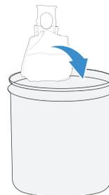
\* Hold the Handle to lift out the Dust Bag, which can effectively prevent dust leakage.
