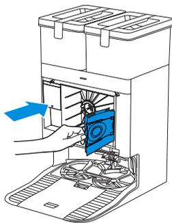
3. Place the fit joints at the upper edge of the Dust Cabin cover and press the lower part of it to install it properly.
