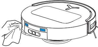
**Note:** Wipe the contacts with a dry cloth. To prevent water damage, avoid using a wet cloth.
