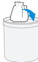
Hold the handle to lift out the Dust Bag, which can effectively prevent dust leakage.
