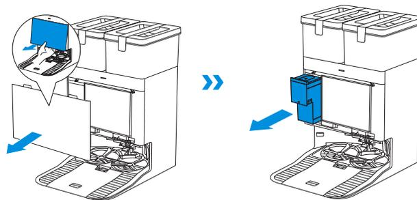
2. Unlid the cleaning solution unit and fill it with ECOVACS Cleaning Solution (sold separately). Put the lid on and the unit back to the Station.
