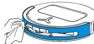
**Note:** Clean the sensor lens and the Bumper with a dry cloth. To prevent water damage, avoid using a wet cloth.
