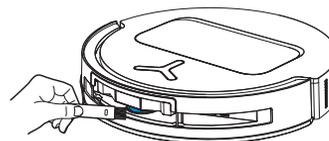
**Note:** Rotate the Module lens to the front and clean it gently with a soft brush.
