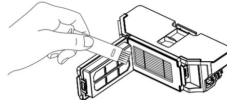
4. You may wash the Dust Bin and the Filter with running water. Shake off the remaining water from the parts.
