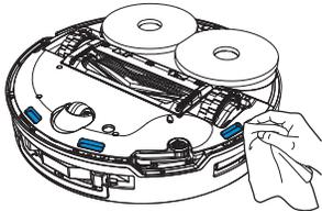
**Note:** Clean the sensor lens and the Bumper with a dry cloth. To prevent water damage, avoid using a wet cloth.
