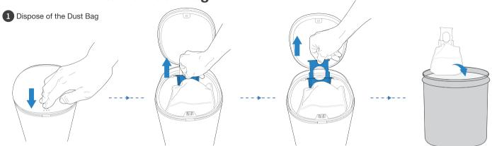
\* The Dust Bag will be sealed by the handle so the dust will not leak.
