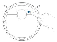
**Note:** The robot's Control Panel stops glowing after the robot is paused for a few minutes. Press the AUTO Mode Button on DEEBOT to wake up the robot.
